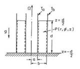
Diagram of fluid annulus  $(r,\phi,z)$  are cylindrical polar coordinates of a point P, fixed in a frame which rotates uniformly with the annulus at  $\Omega$  rad.sec<sup>-1</sup>.  $\Delta T = T_b - T_a = 4$  or  $10^{\circ}$ C. a=2.5cm, b=8.0cm, d=14.0cm,  $0<\Omega<5$  rad.sec<sup>-1</sup>.
